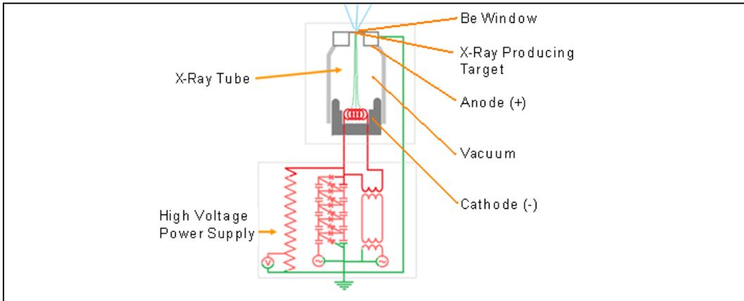
The current applied to the filament changes the intensity of the X-ray by changing the number of electrons emitted from the miniature coiled tungsten filament. More current means more electrons.
