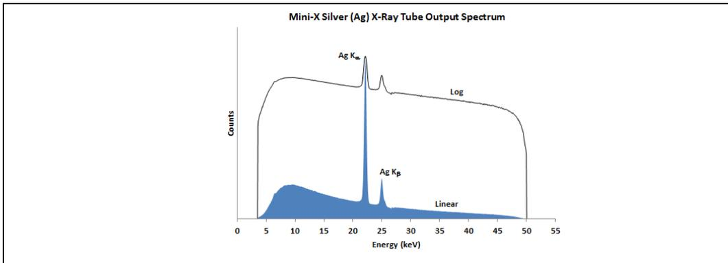
X-Ray production voltage and current settings in the handheld XRF Analyzer has been programmed to produce the energy and intensity required to obtain the best analysis results for a particular application. The user does not make any voltage or current adjustments in operating the XRF analyzer.
