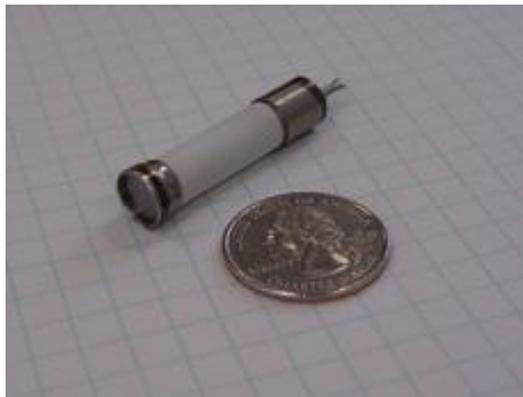
A current passed through a miniature coiled tungsten filament raises the temperature of the wire to approximately 1000°K, causing the thermionic emission of electrons. Typical currents of 5 to 100  $\mu$  amps of current are used depending on the type of analysis being conducted.
