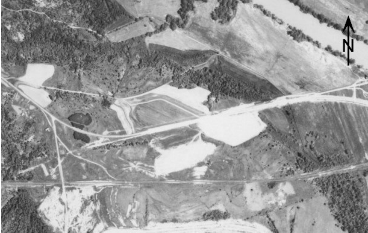
Figure 1.6. Aerial photograph showing the Ayers Town site area in 1959, during construction of the SC Highway 5 bridge and approaches. The site boundary is shown in red; the white areas west and south of the site indicate extensive soil removal. Photo 1959-PL-3W-238; courtesy of Chad Long, South Carolina Department of Transportation. (Site location removed)
